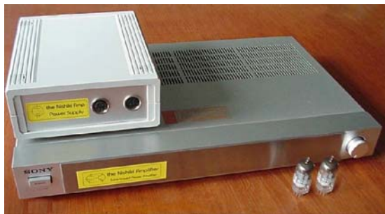
Fig.14 The Nishiki Amplifier using a Sony enclosure and external PSU
